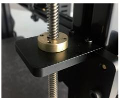
4 bolt locking thick bushing enable better linear track.
